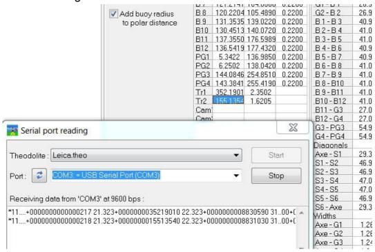
With Leica TC models, after download, you may see a message on the theodolite screen which says 'Communication failure'. This is because there has been no acknowledgement but it is not a problem. Press the red button to clear this and carry on. With Flexline instruments you can turn off the acknowledge signal. This means that you no longer get the error message. Go to Menu>Settings>Interface and on the second page there is an option for Acknowledge on or off. Turn it off. (see bottom of page)
